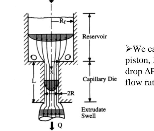
We can record force on piston, F (or the pressure drop  $\Delta P$ ), and volumetric flow rate, Q
