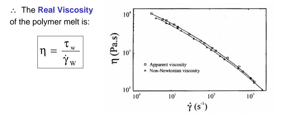
>To obtain the "true" shear rate we must plot Q vs  $\tau_w$  on logarithmic coordinates to evaluate the derivative dlnQ/dln $\tau_w$  for each point of the curve
