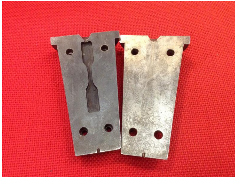
Figure 6. Dog bone mold, for mechanical test samples.
