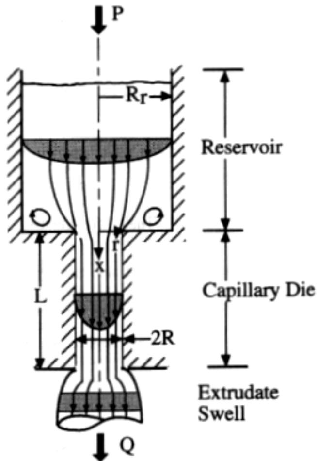
➤ We can record force on piston,  $F$  (or the pressure drop  $\Delta P$ ), and volumetric flow rate,  $Q$
